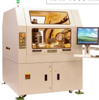
Providing the link to automated End of Line processing, the **IDM1000** inline PCBA dicing system complete with board handling.
