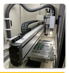
The GSR1200E is a single table standalone router machine that is specially designed to route (de-panelize) large panels with PCB size up to 500mm x 450mm into individual units. It is capable of speeds of up to 100mm/s and positioning speeds of 1000mm/s. The superior servo axis system provides high acceleration/deceleration, reducing cycle time (increase in production output) and at the same time maintaining high accuracy cutting.
