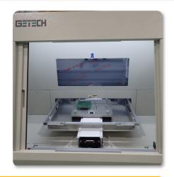
The GSR1280E is a single table standalone router machine that is specially designed to route (de-panelize) large panels with PCB size of 610mm x 610mm into individual units. It is capable of speeds of up to 100mm/s and positioning speeds of 1000mm/s. The superior servo axis system provides high acceleration/deceleration, reducing cycle time (increase in production output) and at the same time maintaining high accuracy cutting.
